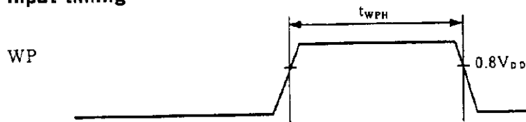
Fig. 7 Wake-up input timing
